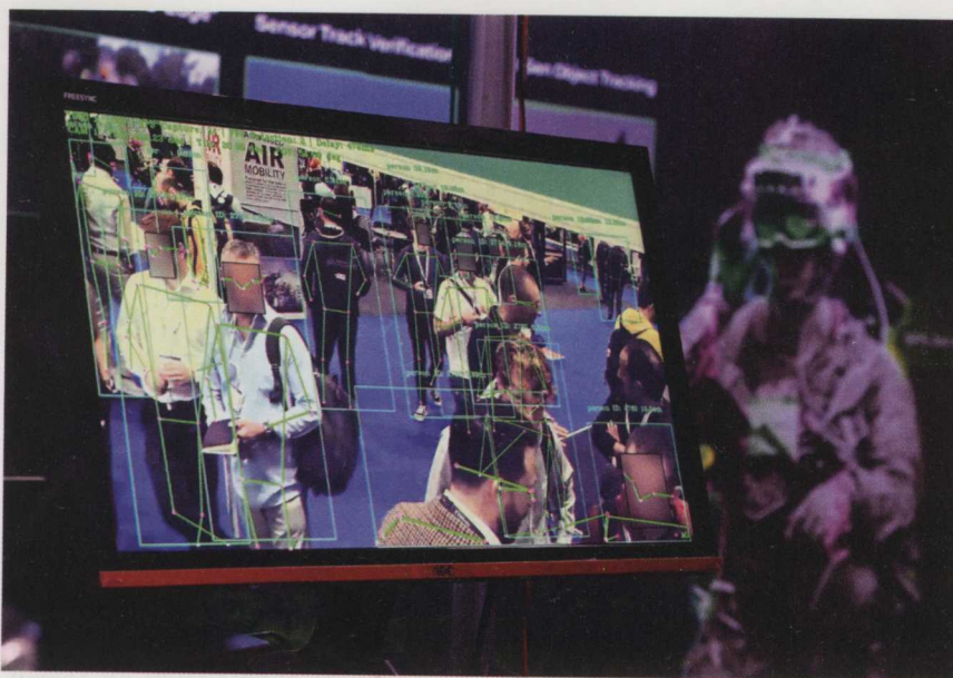
The Vizgard FortifAI software-based AI engine for surveillance monitoring is displayed on September 26, 2023, in London, England. The system operates face redaction to avoid non-compliance with regulations by anonymizing faces and license plates with a real-time redactor. The AI engine integrates with camera-based security systems and unmanned platforms to reduce operator burden and increase the probability of detecting potential threats by recognition of basic human physical behaviors such as walking, running, climbing, crouching, or crawling. JOHN KEEBLE/GETTY IMAGES
