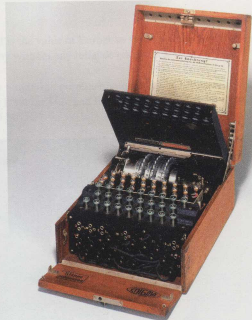
The Enigma machine was patented in 1918 by the German engineer Arthur Scherbius and produced commercially from 1923. The German government, impressed by its security, acquired the rights to the machine and adapted it for military use. Throughout World War II, Germany and its allies encrypted military messages using Enigma machines, and by 1945 over 40,000 were in use. The Germans considered the Enigma code to be unbreakable. However, thanks to combined Allied efforts, the codebreakers at Bletchley Park in Buckinghamshire (the British Army's intelligence center) managed to intercept and decipher the code with the help of Colossus, the world's first electronic programmable computer. This feat is said to have dramatically shortened the war. SCIENCE & SOCIETY PICTURE LIBRARY/GETTY IMAGES
